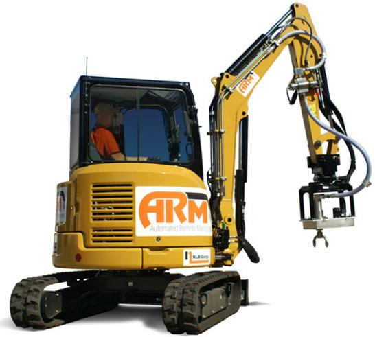
systems with multi-application capabilities. These typically have articulated arms mounted on commercial excavators, with changeable tooling designed to accomplish specific tasks.
