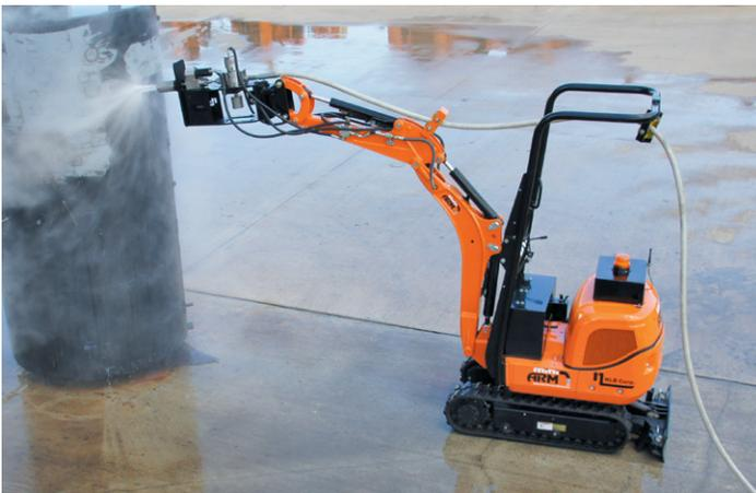
Since semi-automated systems are directed by remote control, or from a cab, they allow operators to keep their distance from the high-pressure water and any flying debris. This exposes the operator to less risk (and fatigue) than holding a high-pressure lance and makes it easier to comply with OSHA personal protective equipment (PPE) requirements.
