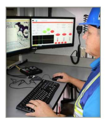
Modern look and feel; displays packer pressure, sleeve vacuum/pressure, pump speed, daily and per joint totalizers.
