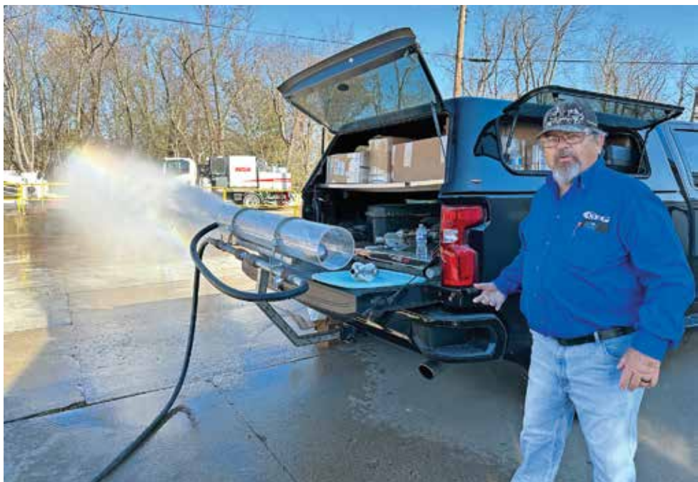
▲ A high-efficiency Tier 3 nozzle running 60 gallons a minute at 2,000 psi will impact debris 9 feet away with 98 pounds of force.
