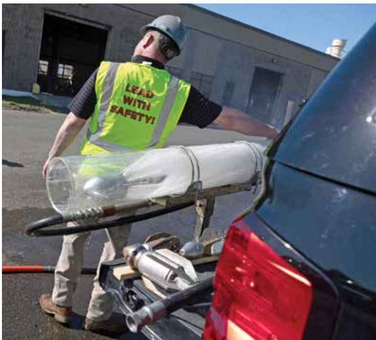
📌 Tier 3 nozzles can deliver safer sewer cleaning at lower psi.
