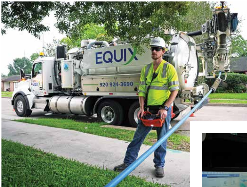
◀ Bryce Elliott, jet/vac operator, retracts the hose on a 2023 KAISER AquaStar during a job in Houston.
