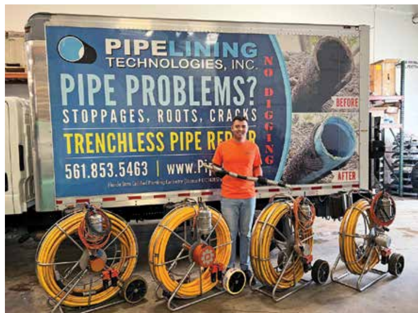
▲ Loren Wilson, operations manager for Pipelining Technologies in West Palm Beach, Florida, stands behind four of the company's Dancutter DC Super Flex robotic cutting machines.
