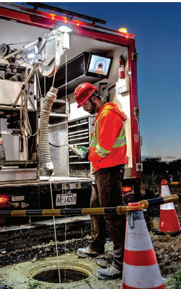
« A technician operates the controls of an IBAK inspection system.
