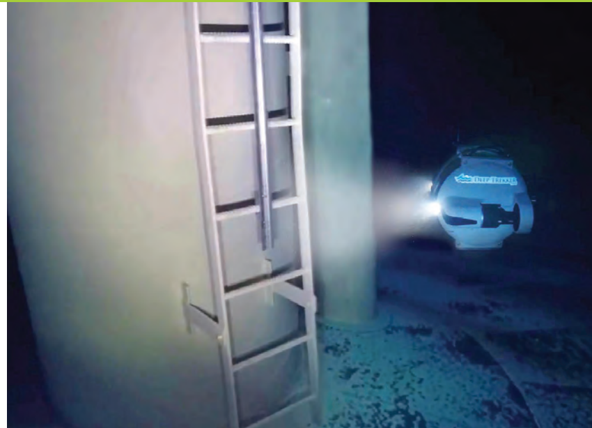
▲ The Deep Trekker submersible drone camera, shown here in a water tower, can “fly” through water via remote-controlled thrusters and dive as deep as 500 feet.
