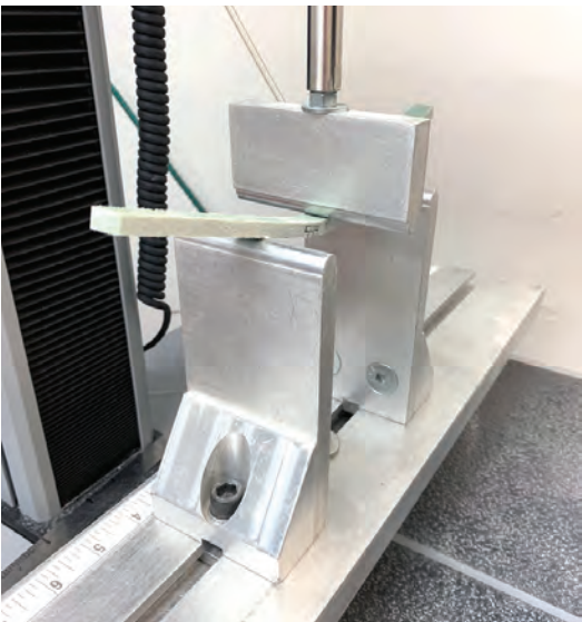
⤴ The ASTM D790 flexural test of a standard felt liner sample.
