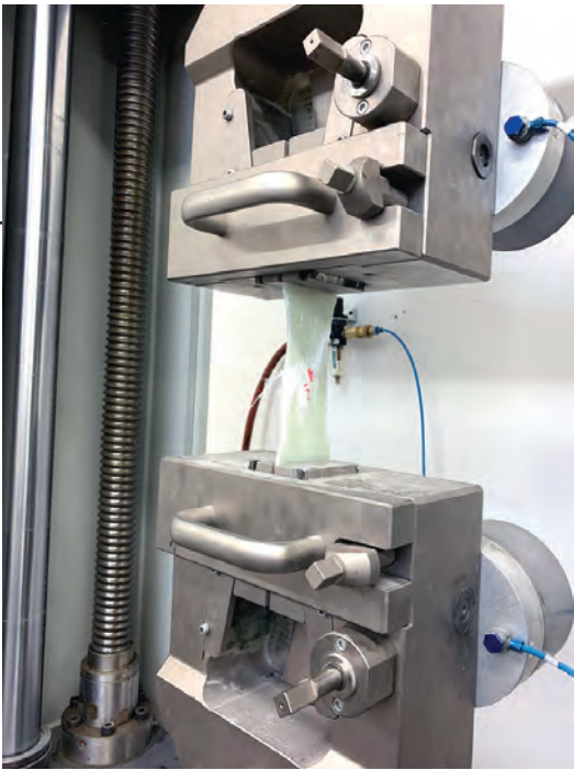
⤴ The AST D638 tensile test of a 2-inch-wide fiberglass liner sample in accordance with the City of Los Angeles Greenbook.
