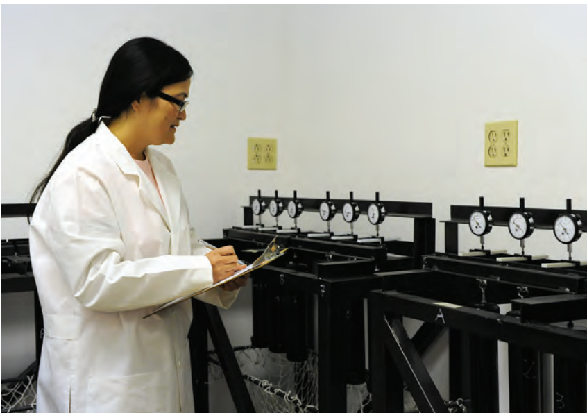
◀ HTS Pipe Consultants lab manager Khamla Phouangsavanh records ASTM D2990 flexural creep test deflection measurements of a felt liner sample.
