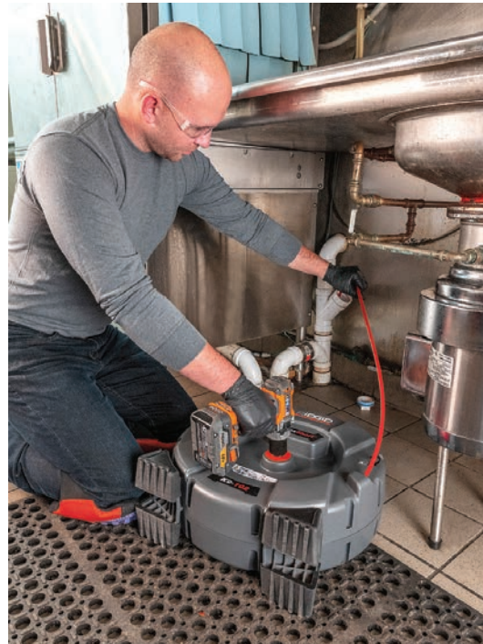
With Flexshaft machines, like the RIDGID K9-102, the cable spins about four to five times faster than traditional cable machines, using low torque and high speed to clean wall to wall in the pipe.
