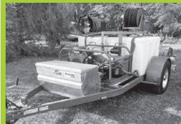
**2014 FNA tow behind Hydro Jetter** and pressure washer system. 250-gal tank. 200-foot jumper hose. 3 reels ranging from quarter inch hose up to half inch hose. 200-foot of quarter inch Jetter hose. 300-feet of half-inch Jetter hose. 150-feet of 3/8 Jetter hose. 3400 PSI at 7-8 GPM Honda motor, head kits, foot pedal. Extra tools and equipment included. Well-maintained. .... Asking \$14,500
