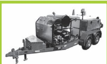
**The HotJet II®** is a best-selling hot- and cold-water drainline cleaner featuring a 35hp Vanguard engine by Toyota and delivering 10gpm @ 4,000psi that cleans drains up to 300' and 12" in diameter. Priced at \$39,995 the HotJet II® is American made using nonproprietary parts for affordability and ease in serviceability making its return on investment truly impressive. Prices subject to change. Financing available.
