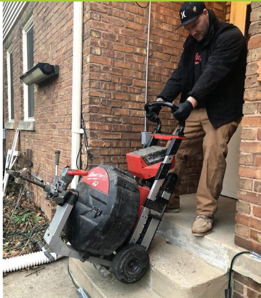
▲ Drains R Us of Southeastern Wisconsin technician Kenny Szczesny guides the Milwaukee Tool MX Fuel drum machine with POWERTREDZ stair-climbing lift-assist technology into a customer's home. (Photo by Ken Wysocky)
