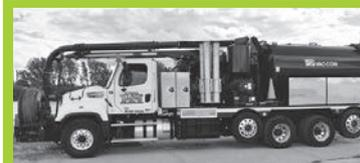
**2019 Freightliner 114SD.** DD13(450HP). Allison 4500RDS Roots Blower 827@18". Water pump 80GPM/3000PSI. 10-YD Debris tank water capacity 1250-gallon. 2 Pressure hose reels. 800-FT JET hose. Build sheet available on request. .... Asking \$317,000
