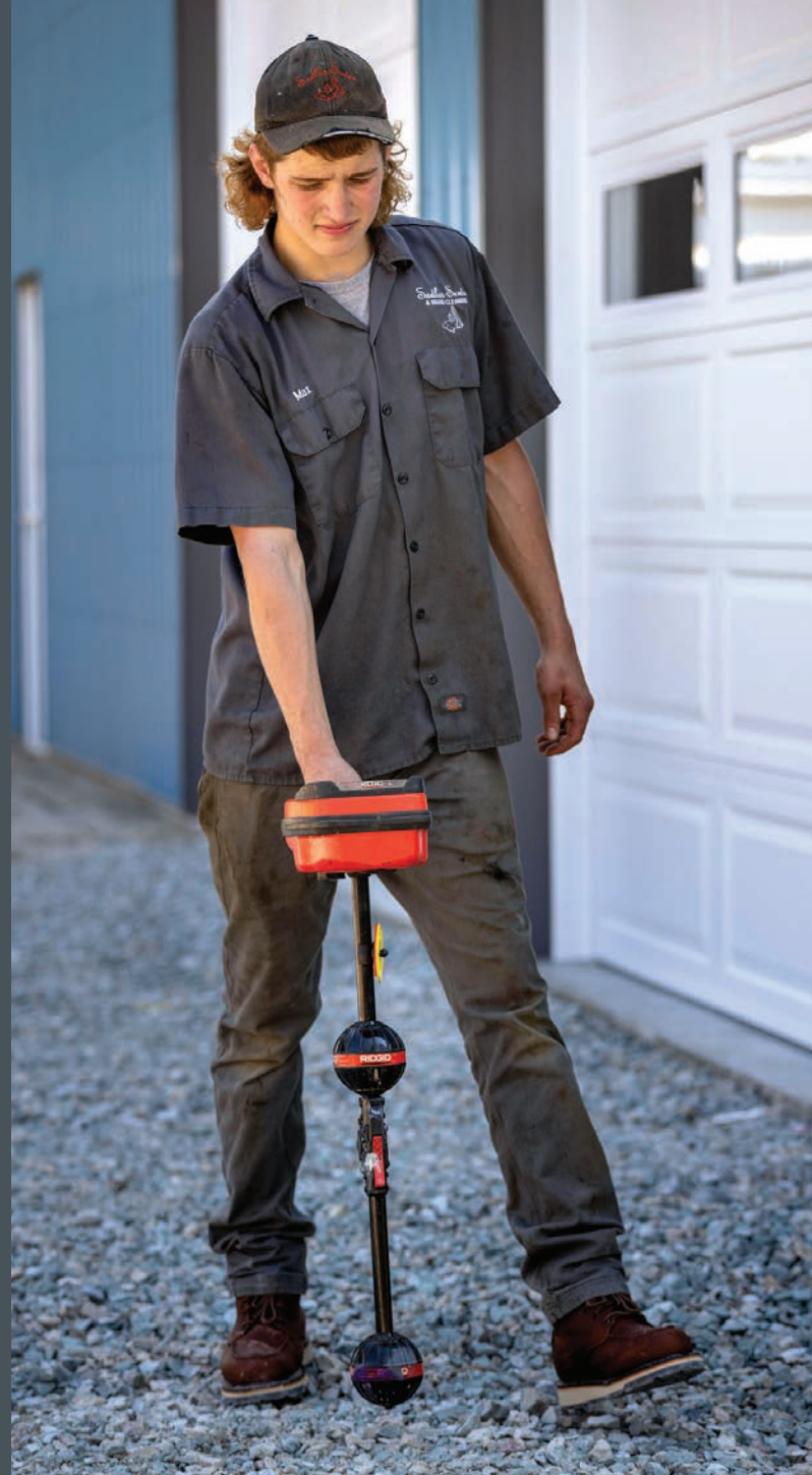
Max Sadler searches for a sewer line with a RIDGID NaviTrack Scout locator.
