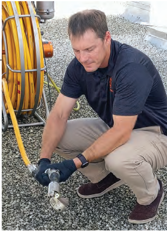
▲ Craig Underwood demonstrates the Dancutter Super Flex. The robotic reinstatement cutter's ability to navigate around multiple bends and one-person operation make this APEX's top pick for CIPP installation.
