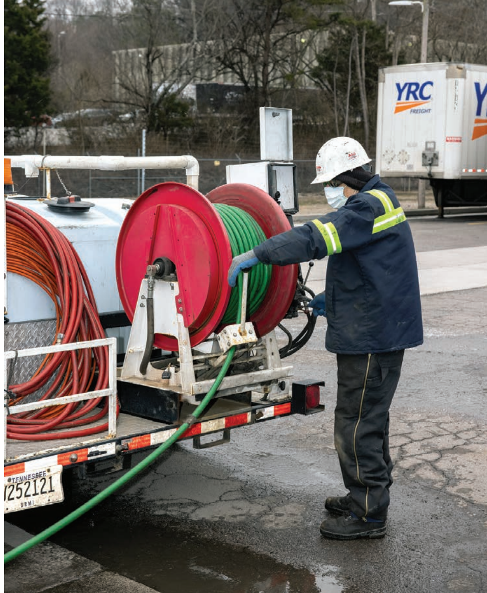
David Kutzer mans the controls of the team's US Jetting 3025 jetter, using a 1/2-inch hose and sand nozzle.
