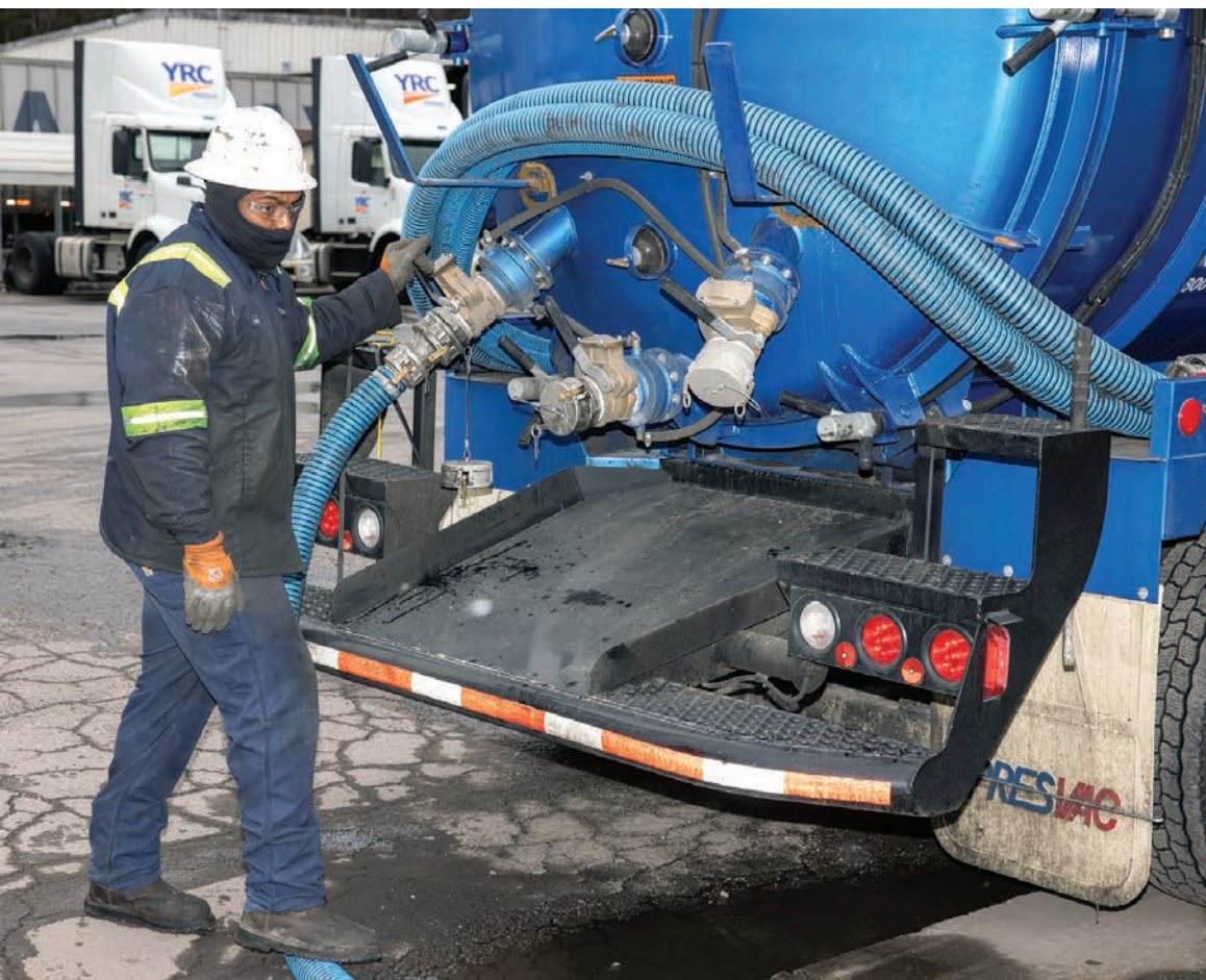
« James Robinson runs a PresVac vacuum truck with an NVE 4307 blower on an industrial cleaning job.
