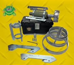
SRRK-1 Super Green Meanie Green Kit The round profile allows the cutter to enter sewer lines 4" and up. Motor handles flows from 40 - 80 GPM and pressures 2000 - 3000 PSI. Rated up to 235 ftlb. of torque, and 175 ftlb. of continuous torque. Kit comes with SRRC-1P Super Green Motor; 1" Saw Blade Hub; 6", 8", 10", 12" HD Concave Saw Blade; 6", 8" Cage Skid Single Size; Set Of 10" & 12" Fins. Motor fits Green wheeled skids you may have.
