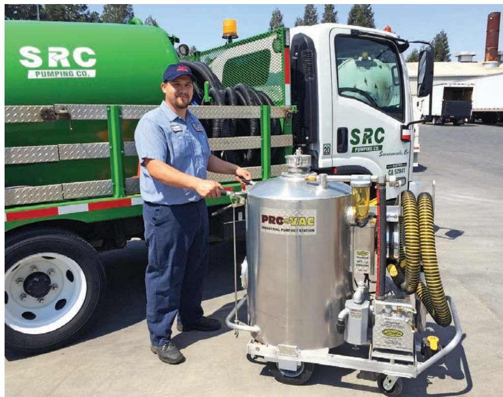
➤ Ray Castro, a technician with California-based SRC Pumping, wheels a Conde ProVac portable pumpout unit into a job. The company uses the machines for pumping grease traps in cramped kitchen areas.
