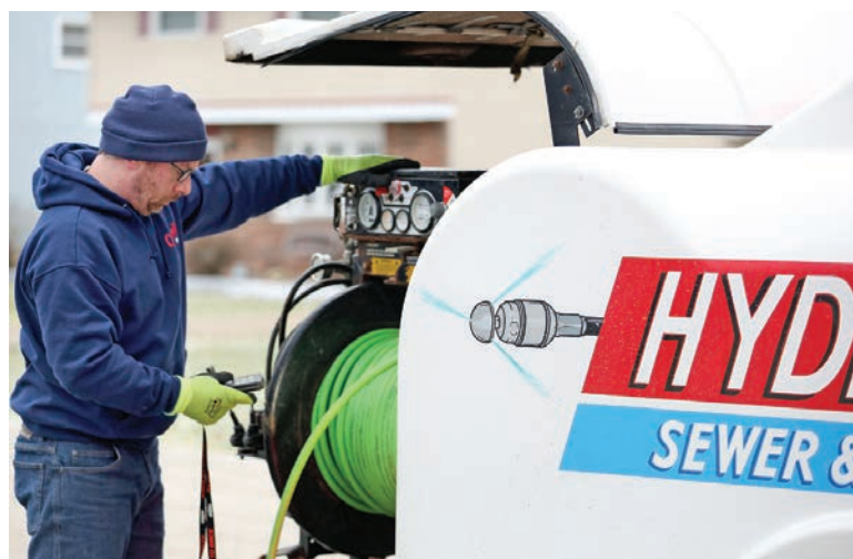
Technician O'Brien sets up a 2015 Spartan Warrior jetter (above) to clean a later line (below) at a home in Eastlake, Ohio.
