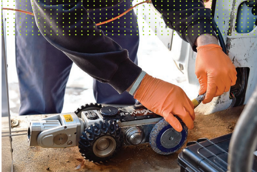
🚚 Zach Gleoge sets up a Rover X for a sewer inspection.
