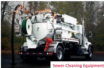
Sewer Cleaning Equipment
