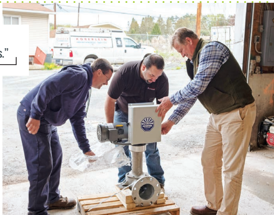
Gene Mohrmann (left), Mike Sprague and Chris Ravenscroft look over a Purestream comminutor prior to installation.
