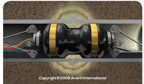
An air-pressure test detects a failed joint, which is then sealed by grout pumped to the packer. The grout flows through the leak, sealing the soil to form an impenetrable barrier.
