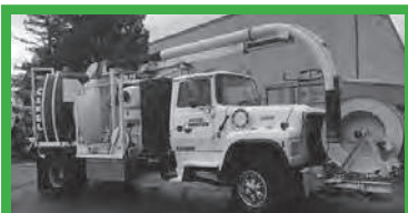
1995 Ford L8000 combination truck - 90,867 miles, 40,000 GVW, 6-yard debris tank, 1,500-gallon freshwater, Myers D65-20 pump, 65gpm @ 2000psi. Roots 800RCS Series blower. 8" suction, 600' 1" sewer hose. Excellent condition. .... $28,000 Call 415-898-2700, CA C10
