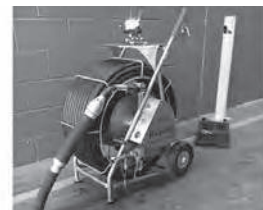
IMS Micro Automatic Plus , air-powered lateral cutter, 3"-10" line capability, joystick control for drive/lift/rotate, 164" hose length. Like-new, only used a few times. .... $57,600
