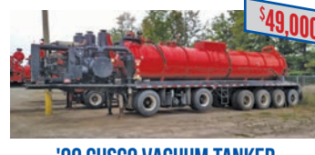
'90 CUSCO VACUUM TANKER (162) Self-contained, 6 axles, blower/vane, 5500 gal., twin disc clutch, 6B Cummins, full open rear door
