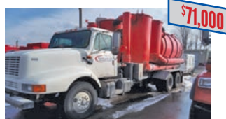
'99 INTERNATIONAL/GUZZLER DRY VAC (916) Cat C-10, 8 spd, Roots 1021 blower, Guzzler dry vac, ½ open rear door
