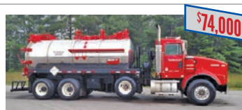
'96 KENWORTH/PRESVAC (920) Cat 3406, 13 spd, 3,500 gallon, full open rear door, NVE Challenger vacuum pump
