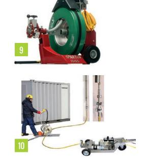
optional power feeder. It comes with a standard configuration of 150 feet of 11/16-inch hollow-core cable, which should reach most blockages with a single reel. It weighs 185 pounds, and adding a loading ramp and electric winch to any vehicle makes transportation quick and simple. It is designed to clean pipes from 3 to 8 inches in diameter. 877-446-7548; www.gorlitz.com.
