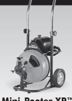
Mini-Rooter XP™ Basic Unit – No cable cutters or power feed
