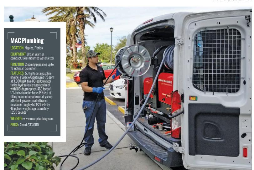
80-gallon water tanks; a hydraulically operated reel that pivots 180 degrees and holds 460 feet of 1/2-inch-diameter hose; 155 feet of filling hose; automatic run-dry shut-off; and a steel, powder-coated frame. Its dimensions are roughly 52 1/2 by 49 by 47 inches, and it weighs approximately 1,200 pounds. Carestia opted to pay extra for an optional remote control and a footage counter.
