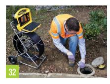
output, keyboard input and a condenser microphone with an on/off switch. It has a high-resolution, low-lux color camera; AC/DC input; keyboard for annotation; video/audio output; microphone; and is fully locatable with 512 Hz in-line transmitter. 800-767-1974; www.rstechserv.com.
