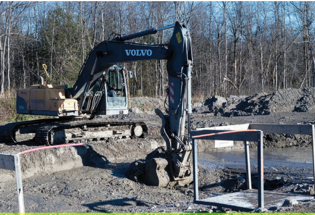
Water and dirt get separated for reuse after hydroexcavation spoils are dumped at NCM's eco-friendly waste facility.
