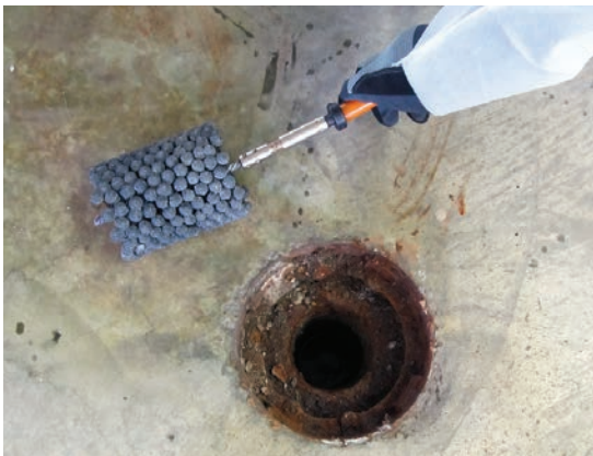
▲ The Little WIZARD scrapes debris off pipe walls via high-torque, high-speed rotation of various scouring heads/tools.
