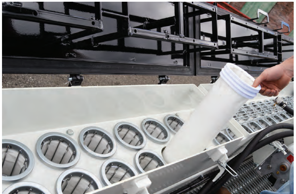
Filter bags in the baghouse are checked from the top of the hydroexcavator.
