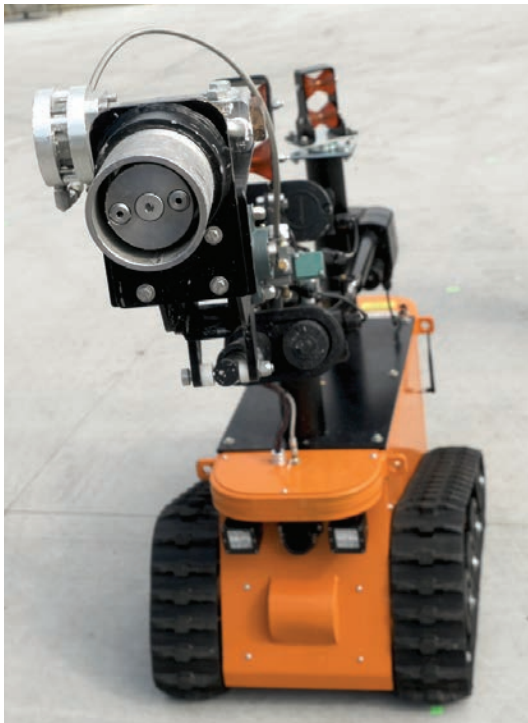
The robotic hydro blasters are easily positioned for cleaning jobs. Tracks with rubber treads allow the machine to climb stairs and navigate narrow catwalks.
