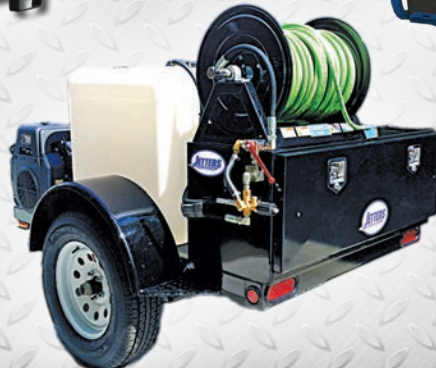
Brute 150 150 gallon, 9 gpm, 4000 psi
