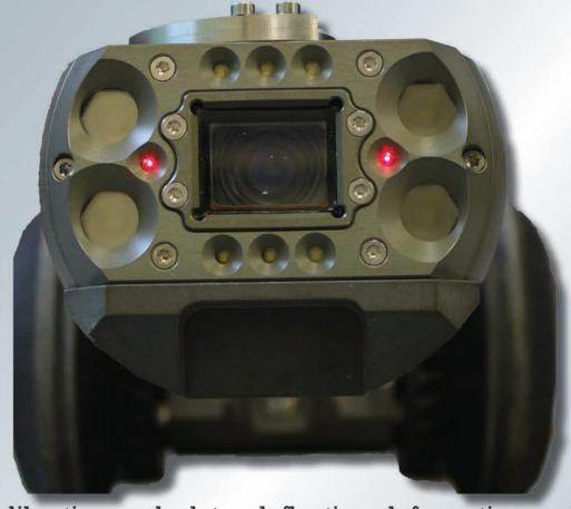
no field calibration • calculates deflection, deformation, and diameter laser crack measurements
