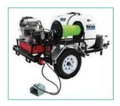
front jack with wheel, safety chains and aluminum fenders. The jetter includes a Honda GX690 twin-cylinder electric-start engine, V-belt drive, trailer-mounted skid, and 15-gallon EPA- and CARB-approved poly fuel tank. Its TS-Series General triplex plunger pump supplies 8 gpm at 3,500 psi. It has a pumpmounted jetter pulse valve, foot valve with 8-foot jumper hose, and three jetter nozzles — the Penetrator, Flusher and De-Greaser/De-Icer. 800/333-9274; www.watercannon.com.
