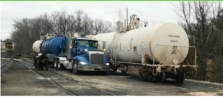
The VacSimizer trailers combine a 5,000-gallon tank typical of a full-size tanker trailer with the smaller size and greater maneuverability of a standard vacuum truck.
