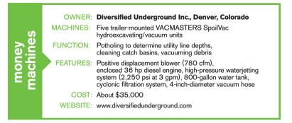
the same is true for a lot of the soil around here, which is usually hard clay or pretty rocky," Allen explains. "We also spec'd 4-inch vacuum hose because it doesn't clog as much as 3-inch hose."
