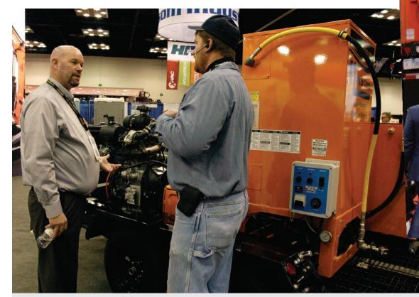
NLB sales representative Kirk Bell (left) points out the features of the company's new 535 Series high-pressure jetting unit to an attendee at the 2016 WWETT Show. The unit features an Epps 700,000 Btu 12-volt diesel-fired heater that keeps water consistently hot for long periods. (Photo by Craig Mandli)
