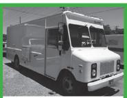
2001 GMC Grumman P31 diesel Pearpoint sewer inspection truck. Complete setup. Two (2) explosion-proof cameras. 19.000 miles on truck, 2.100 hours on Onan 7.5 diesel generator. Excellent condition! ..... \$39,000
