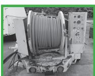
1995 O'Brien swinger jetter, Myers pump recently rebuilt. Powered by a John Deere diesel. 1,500 psi at 40-50 gpm, 3 heads. Hose in fair condition.
