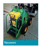
environmentally friendly hydraulic lifting systems produce near zero noise and air pollution, providing the ideal solution for construction sites within city limits or with strict emission guidelines. Hydraulic operation provides improved startup performance in cold weather and eliminates the possibility of fuel freezing in extreme conditions. The hydraulic lifters are lightweight, allowing farther reach and greater total lift capacities. 866/664-3450; www.vacuworx.com.
