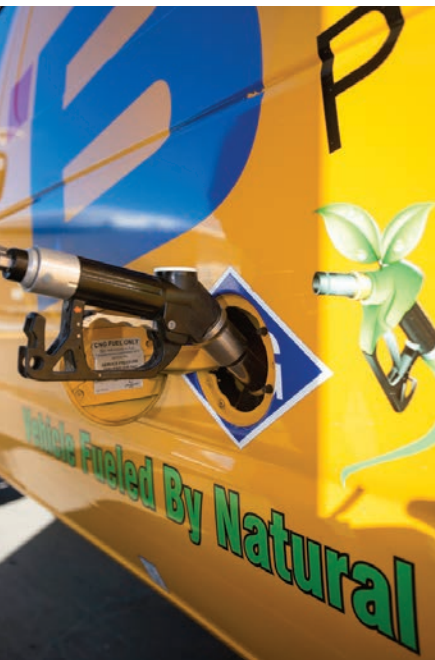
ABOVE: Compressed natural gas flows into one of Backlund's Ford E-250 service vans. Most of the company's fleet has been converted to run on CNG.
