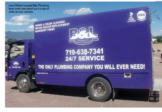
The B&L Plumbing vans feature VT Hackney bodies with customizable storage options and plenty of space for tools and inventory. Each of B&L's vans now carries about \$10,000 worth of plumbing parts, which saves plumbers from making trips to the supply house.
