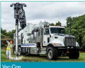
vacuum breaker, dump controls and hydraulic door locks from remote areas up to a half mile away. The boom rotates up to 270 degrees. **855/336-2962**; **www.vac-con.com**.
