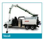
muddy clothing. The compartment has floor drainage, racks to hang dry clothing, heated cabinets for the hose reel and water pumps, and boilers that can heat water for more effective hydroexcavation in frozen ground. The unit uses high-pressure jetting action to loosen soil, rocks and clay, then strong vacuum (up to 27 inches Hg and 5,800 cfm) to remove the material and water slurry into a debris tank. **800/382-8302; www.vacall.com**.
