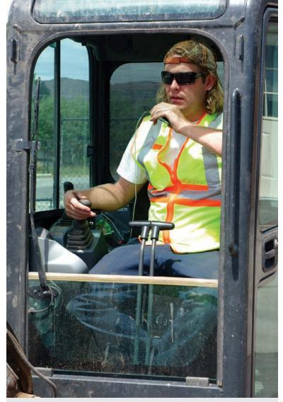
Ron Smiley operates the company's mini-backhoe on a pipe bursting project. The pipe bursting equipment runs off the backhoe's hydraulics.
