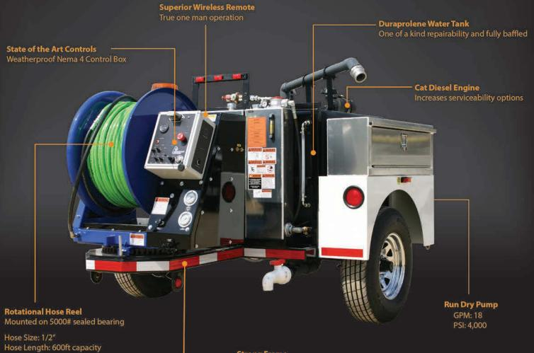
**Strong Frame** Made from tubular steel for superior durability
