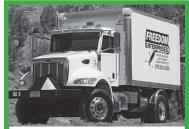
**2011 Peterbilt** custom-built jetter/waterblaster truck. A one-of-a-kind truck that has it all. Cummins PX8 330hp, 13-speed Eaton-Fuller transmission, Jetstream 3000 Series pump 25gpm @ 15,000psi. 925-gallon heated water tank. 1,500 ft. hose reel on 3-foot slide-out. Hydrostatic-drive single engine design, 175hp PT0. Cold weather package. 120v pure sine wave inverter, Pro-Heat programmable heater. \$100,000. Please call Melinda at
