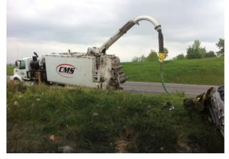
Proper maintenance of you hydroexcavator is critical. If your machine starts to lose suction, don't crank up the rpm, check the filter bags. Blowers shouldn't need anything more than checking and changing the oil at regular intervals.
