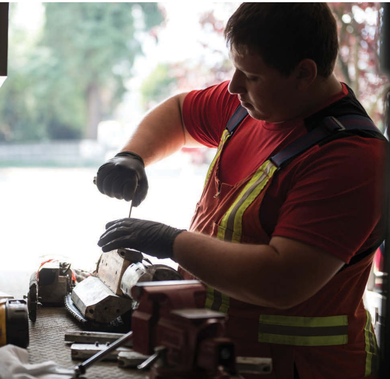
Devlin Hawkes changes the wheels on the camera before a pipe inspection.
