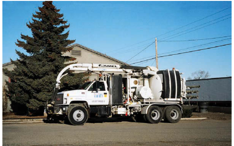
The mid-mounted reel on the Camel 200 combo unit helps Sweet’s Services in Shoshone, Idaho, clean irrigation pipes that aren’t laid to grade and are often accessible only through 4- to 10-foot risers.
