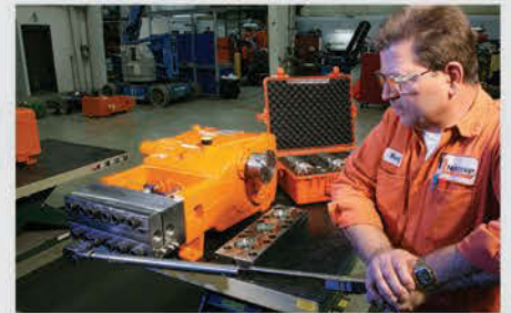
Convert to 40,000 psi in about 30 minutes — faster for lower pressures.
