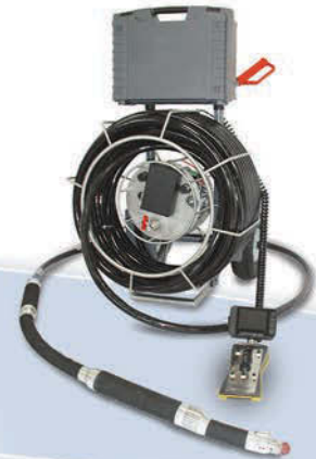
Positioned with remote air bladders, IMS Micro travels 100' into laterals 3-6", maneuvers past elbows, articulates on 2 axes, and views with an illuminated camera.
