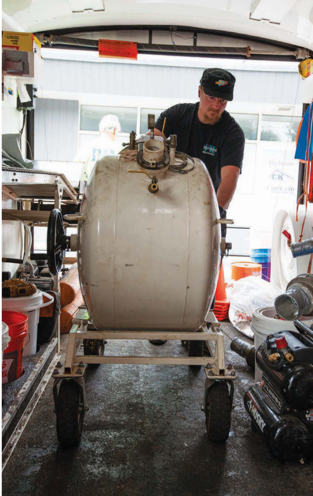
>> RIGHT: Matt Leger moves CIPP lining equipment out of the New England Pipe Restoration work trailer to set up for a lateral lining job.
