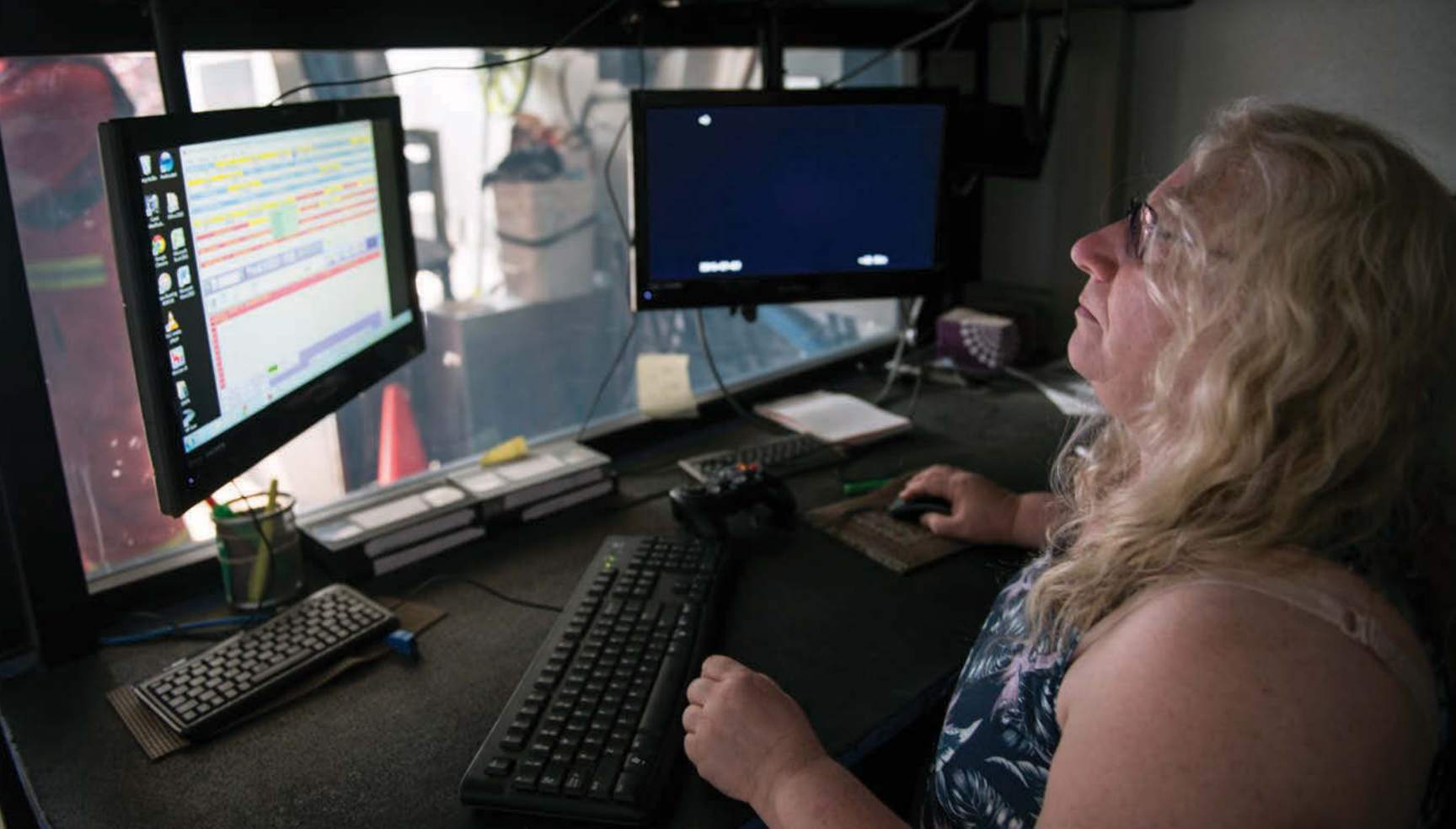
Rosa Hawkes operates a CUES Shorty inspection system from the control room in the TV truck. ABC records, analyzes and delivers inspection videos to clients on site immediately following an inspection.
