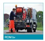
unit is designed for suction and jetting activities. It is ideally suitable for clearing and cleaning house connections and municipal sewers, and the draining of flooded basements and grease traps. It comes with a Speck highpressure pump. The vacuum system can be used with a thrust jetter or a vacuum pump. **www.rombv.com**.
