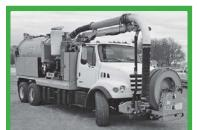
2001 Vac-Con jet vac combo: CAT 3126 engine, Roots 824 PD blower, Allison automatic, 55,000 miles. 600 ft. 1" hose, 2,000psi @ 80gpm, 1,300-gallon water tanks, 12-yd. debris tank. Cummins 4BT rear engine, rear strobes, arrow board on rear. Debris body flush system. 8" telescoping boom. Truck engine over hauled summer of 2014 and newer PD installed fall of 2014. Excellent condition. ..... \$80,000 OB0
