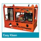
Cat pumps, belt or gearbox drive systems and 12- or 120-volt oil-fired burners. The heating coils are constructed of Schedule 80 or 160 (depending on the model) elliptically wound pipe and concealed in a stainless steel housing. They have a 150 degree F heat rise and a 200 degree F outlet temperature. The fully welded powder-coated steel frame is designed to be trailer mounted for extreme conditions. Gasoline-driven units are also available. 800/315-5533; www.easykleen.com.
