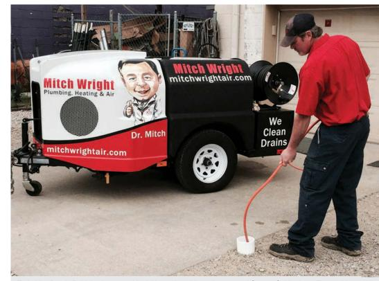
Technician Ronnie Baldwin cleans a residential lateral line with a trailer-mounted Spartan Soldier jetter. The machine has quickly become a significant profit generator for Mitch Wright Plumbing, Heating & Air in Southaven, Mississippi.
