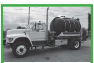
**1998 Camel CJ1600** jet truck: 6,712 hours, 52,021 miles. New water tank in 2013, new water pump in 2012. 50gpm/3,000psi. 3/4" x 600' sewer hose. Ex-city unit.
