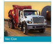
positive-displacement blowers are capable of pulling material as much as 700 feet. It is available with a hydroexcavation package that adds a powerful, highpressure water system that works together with the vacuum system to effectively excavate around sensitive underground utilities, locate underground systems and excavate in areas with limited access. 855/336-2962; www.vac-con.com.
