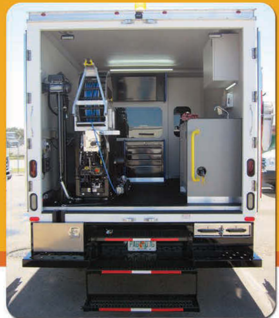
TV Mainline / Lateral Inspection Vehicle
