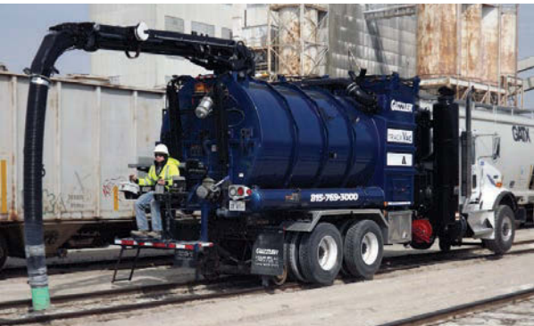
When the truck is in full rail mode, its two front tires are completely off the tracks while two of the rear wheels touch the tracks and bear a portion of the truck’s weight. The operator sits behind the debris body, which increases visibility and safety.
