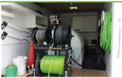
The truck-mounted Cam Spray system features an Udor U.S.A. pump (18 gpm at 4,000 psi), a 49 hp HATZ Diesel engine and a 325-gallon water tank.
