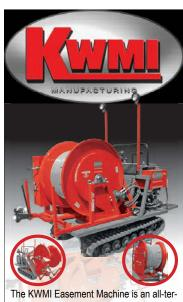
rain rubber tracked power carrier designed specifically for the pumper-cleaner industry.
