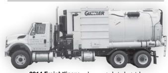
2014 Freightliner truck mounted, industrial wet/dry vacuum loaders with 27" Hg blowers
