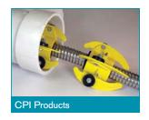
the optimal spot along the camera head or spring push cable. Each section of the skid has four rocking SeamLeapers that swivel back and forth and adjust to various radiuses in the pipe, allowing for wheel contact and maneuverability. It allows for most standard push camera systems to negotiate traps, bends and corners in 4- to 6-inch pipelines while centering the camera at all times. 413/443-0925; www.cplasproducts.com.
