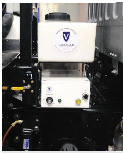
The Vanguard System is designed to disinfect jetter hoses as they're retracted from sewer lines. The system is operated by a truck-mounted control box that combines a cleaning solution with water from the truck's tank.
