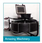
coated lay-flat frame with upright rolling stand; a 1 3/8-inch O.D. metal camera housing; nine dimmable high-output 5 mm LED lights; high-resolution color camera with a self-leveling head; scratch-resistant sapphire glass lens; highgrade 512 Hz sonde locator with an average range of 12 to 15 feet; and an integrated digital video recorder with remote control, compatible with most standard SD cards. 800/504-7435; www.amazingmachinery.com.
