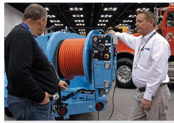
Dean Peake, regional sales manager with Hi-Vac, points out some of the features on the O'Brien 7040-SC dieselpowered hydrojetter's hydraulically actuated reel. The unit features variable-speed control on an easy-to-use control panel. (Photo by Craig Mandli)
