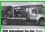
3-stage fan, 12-yd. debris tank, 92,484 miles, 10,541 hrs. Pony motor 2,073 hrs. ..... \$135,000
