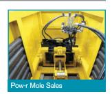
productive. It creates 4,500 ft-lbs of torque, allowing the operator to steer the boring machine up to 200 feet. Quick disconnect hoses allow for fast and easy removal of the unit. 800/344-6653; www.powrmole.com.
