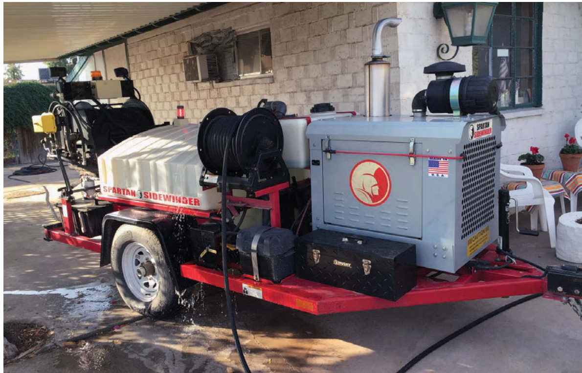
Peerless Plumbing's Sidewinder trailer jetter from Spartan Tool features a Little Giant pump (Franklin Electric) that delivers maximum pressure of 4,000 psi at a peak flow of 18 gpm.
