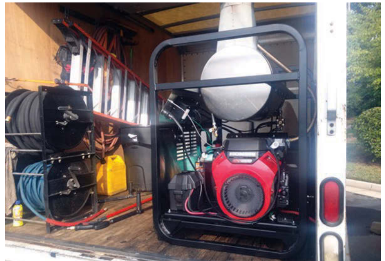
Steam 360° in Leesburg, Va., increased productivity significantly when it switched to Mi-T-M HDS hot-water pressure washers. The company has four units, each with a belt-drive, triplex piston water pump from General Pump, a diesel-fired burner and either a 200- or 400-gallon water tank.
