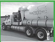
2007 International Vactor 2100: PD 18" blower. 80gpm at 2,500psi with telescoping boom. Hydroexcavation package and trash pump. 1,500 gallons of water and 12-yd. debris tank. International chassis, with 201,000 miles and 8,300 blower hours. ..... \$140,000
