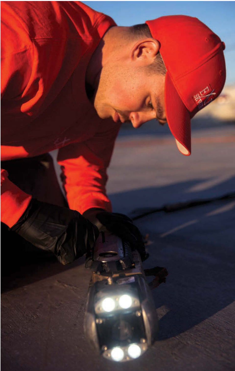
Alan Smith checks over the CUES camera prior to launching it on an inspection job in Rancho Cordova, Calif.
