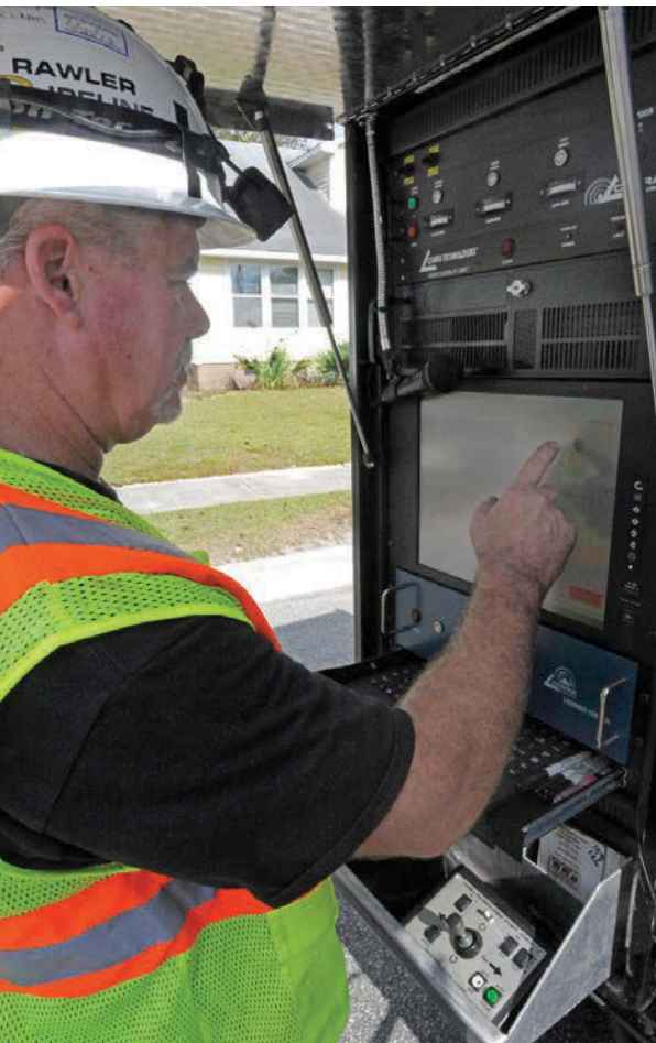
Crawler Pipeline Services Owner Wayne Thompson works the controls of the Cobra Technologies robotic camera.
