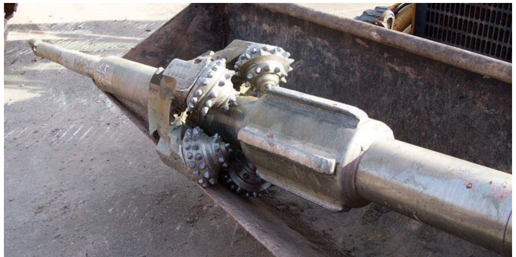
ABOVE: A hydroexcavator from Valley Hydro-Excavation in Campbellspport, Wis., helps a Waas vacuum tank trailer pump drill fluid from the exit pit. RIGHT: The custom-built 20-inch rock reamer has six carbide Tri-Cone bits with large cone offsets, chisel-shaped inserts, and irregular tooth spacings. Fins ahead of the reamer keep it centered in the smaller hole.
