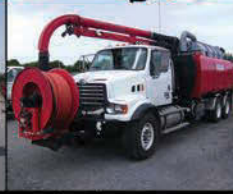
Combination Sewer Cleaner Vacall AJV 1015
