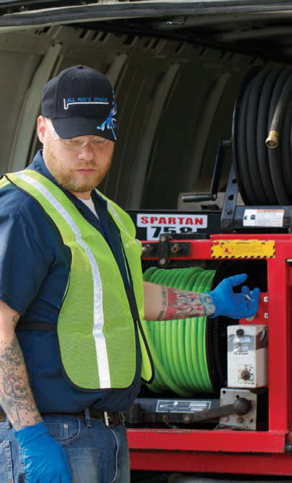
Rich Gilbert operates the controls of the truck-mounted Spartan 758 jetter on a cleaning job.
