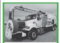
2009 Sterling Vac-Con VPD3616LHAEN S\N: 09085083. Bean jetting pump. Roots 824 RCS blower. 16-yard debris tank. ISX Cummins diesel. Push-button automatic. 54,587 miles. 66,000 GVW. Hendrickson spring.
