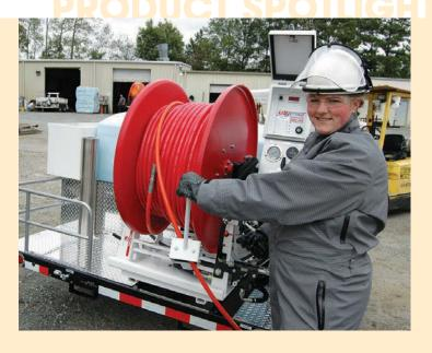
The two-piece jacket with hood and pants provides full body protection to 7,500 psi. The jacket has a detachable hood with room for ear protection, waterproof zippers with overlapping flap, adjustable cuffs and comfort lining. The pants have an adjustable elastic-back waist, detachable suspenders, reinforced
