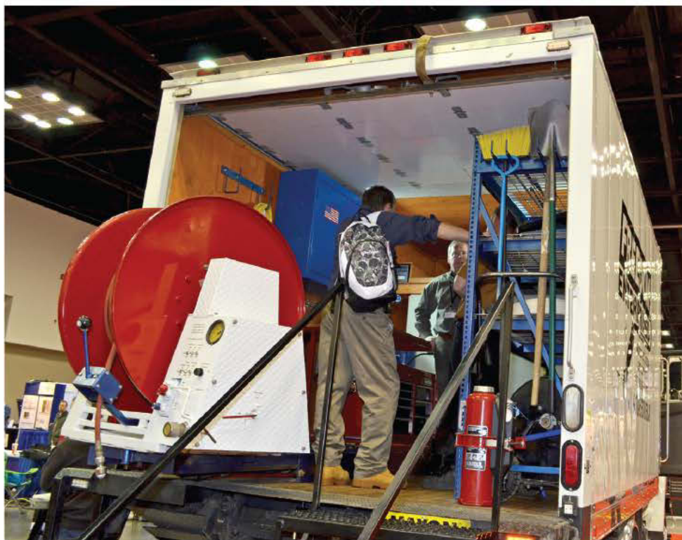
The WBT-3015B water blaster truck from Freedom Enterprises delivers 12 gpm at 15,000 psi or 23 gpm at 8,000 psi. It can also be converted in the field to operate at up to 40,000 psi.
