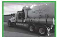
2007 VACTOR 2100 Series: International Chassis, 18" PD Blower, 80gpm at 2500psi,12yd debris tank.
