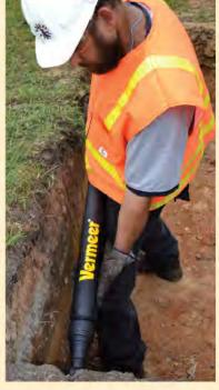
Made of high-grade alloy steel, heat-treated and machined to tolerances of 0.001 inches, the piercing tool is available in 2-, 2 1/2- and 3-inch diameters. The tool's rear tail hose is field-serviceable. Wear rings on the striker and valve reduce steel-on-steel wear. The tool's modular design enables components to be rebuilt, extending its overall life. 888/837-6337: www.vermeer.com.
