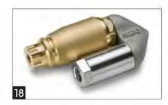
front where they are most effective. The nozzle comes in two 10 gpm speeds (up to 15,000 psi and up to 24,000 psi) and two 20 gpm speeds (up to 15,000 psi and up to 20,000 psi). All models are made of high-grade stainless steel for durability and rotate at 7,000 rpm. They feature an NLB seal design to reduce leakage and can be ordered with four jets for polishing, or five jets for cleaning and cutting. Two more Typhoon nozzles are available for larger pipes. 800/441-5059; www.nlbcorp.com.
