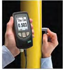
An electronic ultrasonic thickness gauge can test the wall thickness of materials including steel and plastic and determine the effects of corrosion or erosion on any tank structure where access is limited to the outside. (Photos courtesy of DeFelsko)
