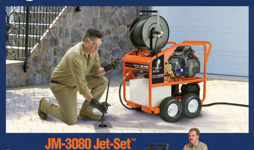
ut trailer jet power where you need it – even in hard to reach places. The powerful JM-3080 blasts grease, sediment and ice from 4" to 8" lines up to 300 ft. long. Tip the trim, precisely balanced jet onto the rear wheels and one person can easily maneuver it into position. Try that with a trailer jet! With a removable 300 ft. capacity hose reel, 20 hp (614 cc) Honda engine and
