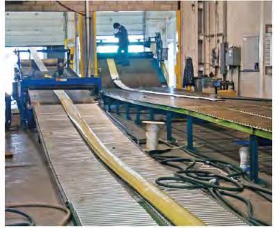
Two production lines of resin-treated liner are impregnated on their way to the loading dock.
