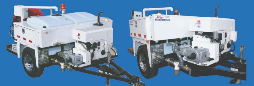
Our US Jetting 4018 - 4000 PSI @ 18 GPM Unit Offers The Best **Cleaning Power In The Industry. Our NEW US Jetting** 6018 - 6000 PSI @ 18 GPM Unit Is Just A Whole Lot Better
