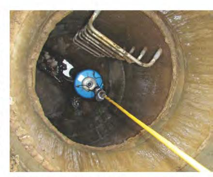
The RapidView IBAK PANORAMO SI manhole inspection camera enables crews to inspect manholes without confined-space entry. (Photos courtesy of PipeTek Infrastructure Services Inc.)
