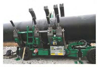
ABOVE: The 1600 fusing machine is the largest made by McElroy. RIGHT: The runway for the HDPE pipe begins at the base of the cliff in the background and the fusing machine is 400 feet from the edge. Aaron Enterprises' fabrication engineer Jeffrey Smith designed the pulling assembly for the new 63-inch HDPE pipe.
