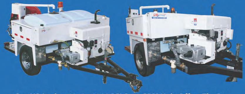
Our US Jetting 4018 - 4000 PSI @ 18 GPM Unit Offers The Best Cleaning Power In The Industry. Our NEW US Jetting 6018 - 6000 PSI @ 18 GPM Unit Is Just A Whole Lot Better
