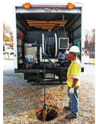
LEFT: An Isuzu box truck carries B. Frank Joy LLC's customized, skidmounted jetter from Sewer Equipment Company of America. The truck also includes a 600-gallon water tank, hydraulic retractable hose reel and an electric jib crane, among other safety- and productivity-enhancing features. ABOVE: Crew leader Santos Romero uses the jetter truck to clean a line. (Photos courtesy of B. Frank Joy LLC)
